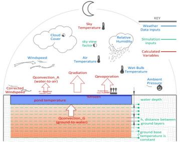
Figure 3. Ice making model features and parameters. "Q" is used to represent heat transfer
