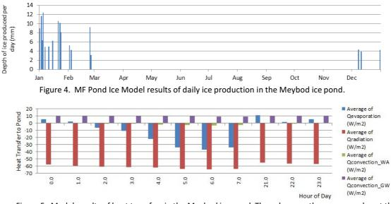
Figure 5. Model results of heat transfers in the Meybod ice pond. The values are the average value at the stated time for all the days of the coldest week.
