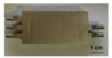
**Figure 4.** Photo of the  $\mu$ MIRHE manufactured in Chromium-Cobalt utilizing the SLM additive manufacturing technique (weighs only 123 g)
