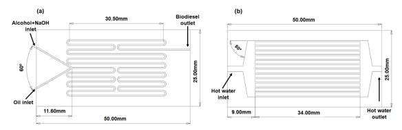
**Figure 2**. Schematic views (a) of the micro reactors layer and (b) of the micro heat exchanger layer.
