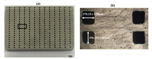
Figure 6. Optical image of the (a) cross section of the  $\mu$ MIRHE; (b) dimensions of the cross sections of the channels
