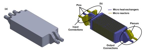
**Figure 1**. Schematic view of the complete  $\mu$ MIRHE showing: (a) the external view of the device and (b) the internal structure of the micro reactors, the micro heat exchangers and the connections (pins and plenums).
