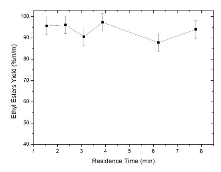
**Figure 10.** Profile of the yield of the ethyl esters (biodiesel) over residence time for the  $\mu$ MIRHE device (cases 2.1 to 2.6 presented in Table 4).
