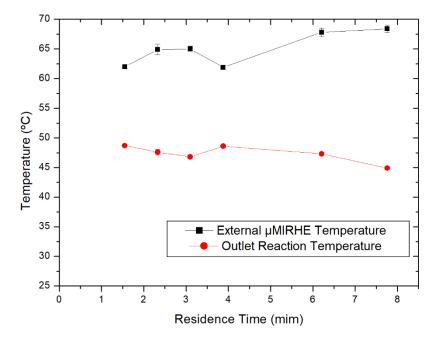
Figure 9. Profiles of the external  $\mu$ MIRHE temperature and outlet reaction temperature
