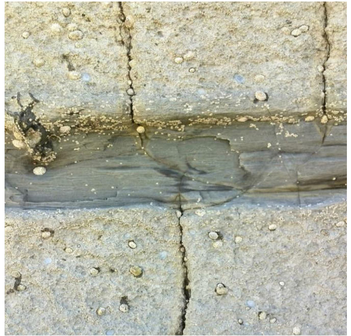
Figure 8. Field work results on limestone and shale layering. Natural hydraulic fracturing in discontinued and inhomogeneous medium.
