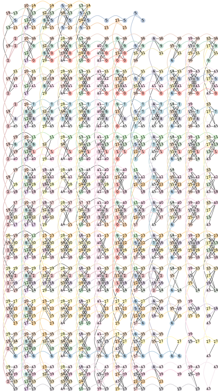
Figure 2.4: Minor-embedding of 46 logical variables into the Chimera interaction graph of the D-Wave 2X. This solution utilises 940 out of 1097 physical variables, that is, 86% of the available qubits. Subgraphs are characterised by the same number and the same colour.
