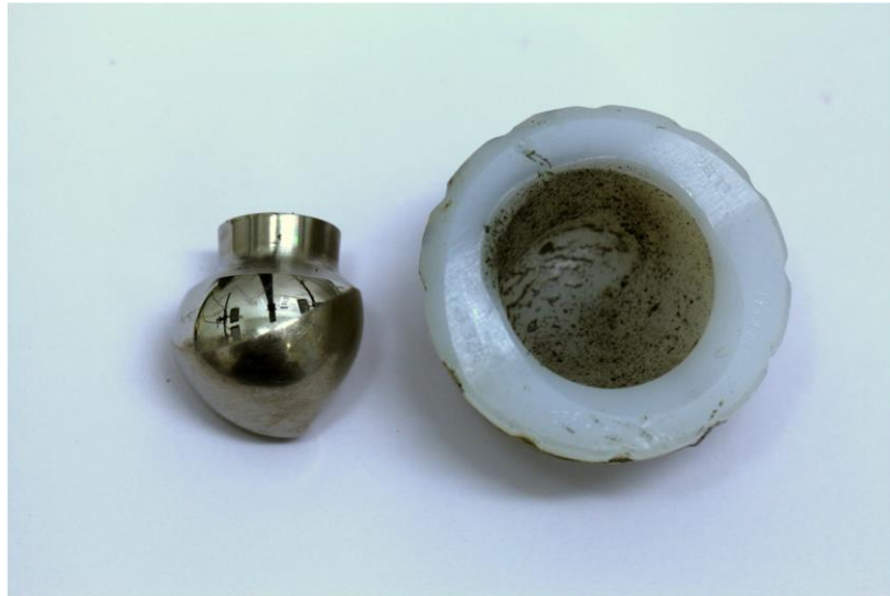
Figure 2.7: The retrieved metal head and plastic cup liner. Substantial deformation of the femoral head can be seen – normally spherical in shape
