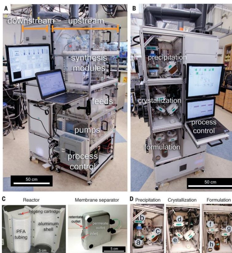
Figure 2-2 Millifluidic system for the synthesis of 4 different APIs, reprinted from Adamo, A., et al., On-Demand Continuous-Flow Production of Pharmaceuticals in a Compact, Reconfigurable System. Science , 2016. 352(6281): p. 61-67, with permission from AAAS.
