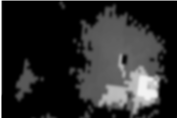
Figure 6: Resource Map (RF signal strength) used in our simulations. The RF signal strength is described from black (no detected signal) to white (highest signal strength). This map was generated with the program cloudf . It uses the Irregular Terrain propagation Model (ITM), also known as the ‘Longley Rice’ model which was designed for planning UHF television broadcasting but has applications across a very wide proportion of the radio spectrum between 20 and 20,000 Megahertz
