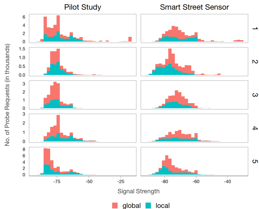
Figure 4.18: Comparison between distribution of signal strengths in probe requests collected by
