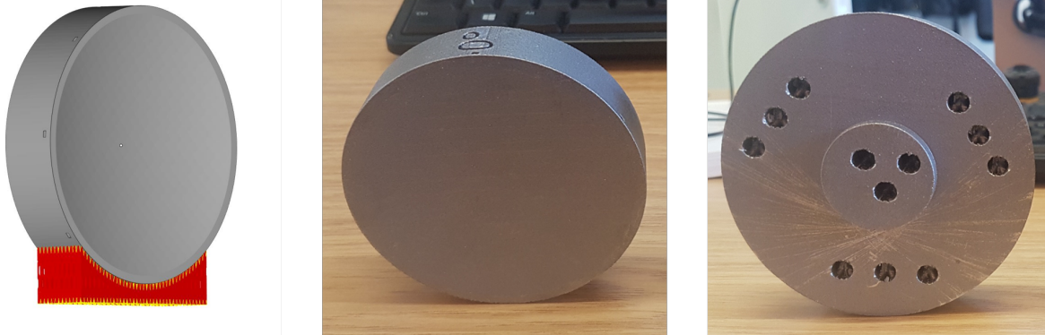
Figure 5. The additive manufacture of the aluminium substrates: left - the design with the AM set-up software where the orientation and the support material (red) is defined; middle and right - the aluminium substrates after printing and with support removal.
