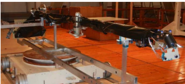
Figure 13. I-Boom installed on a non-magnetic trolley at IABG-MFSA.
