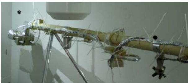
Figure 7. Instrument boom compatibility test at PTB.
