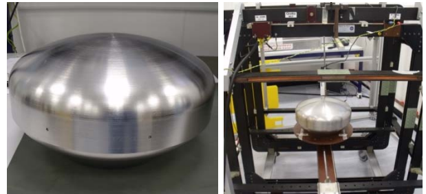
Figure 6. (left) Reaction wheel magnetic shield (right) tested on the Magnetic Coil Facility (MCF) Helmholtz coil in Airbus, Stevenage.
