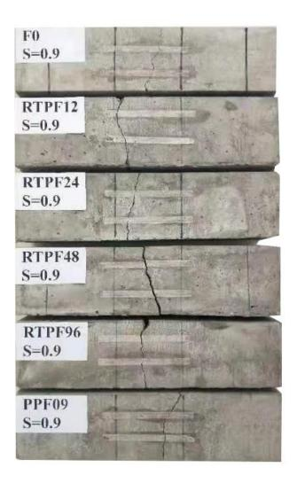
Fig. 18. Failure modes of all mixtures after flexural fatigue loading (S = 0.90)
