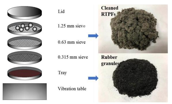
Fig. 3. A schematic diagram showing the process of estimating the composition of RTPF
