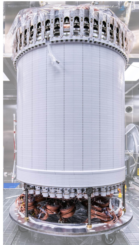
Figure 2: The assembled Xenon Detector. Upper panel labels: 1- Top PMT array; 2-Gate-anode and weir region (liquid level); 3-Side skin PMTs (1-inch); 4-Field cage; 5-Cathode ring; 6-Reverse field region; 7-Lower side skin PMTs (2-inch); 8-Dome skin PMTs (2-inch). Lower panel photo by Matthew Kapust, Sanford Underground Research Facility.
