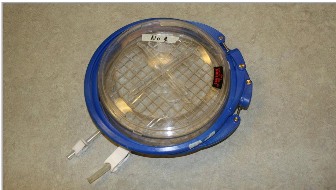
Figure 2.20: Custom-built hypoxic chamber. Plated cardiomyocytes are placed in the chamber, which is then gassed with positive pressure 5% CO 2 -95% N 2 and sealed. The cardiomyocytes are thus exposed to a near-zero Oxygen tension environment, which along with the provision of hypoxic buffer (described in the text) is a well-validated model of tissue ischaemia.
