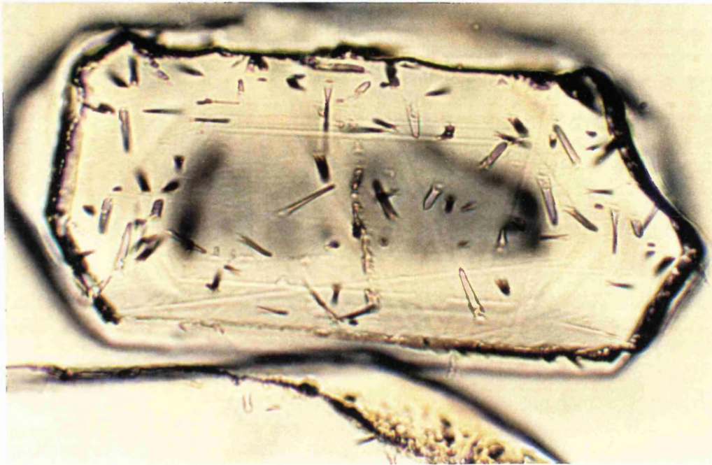
Fig. 7.8. Etched fission tracks in an apatite crystal.
