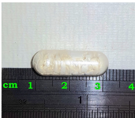
Figure 6.8. A photograph of the coaxial electrospun fibres loaded in a hard gelatin capsule (size 0).
