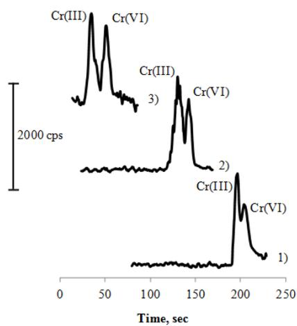
**Figure 3.** Influence of the separation capillary length on the Cr species separation. Sample Cr(III) and Cr(VI) 10 mg/L each; carrier electrolyte 15 mM HNO<sub>3</sub>; flow generating pressure: 1.5 bar; injection time 3 sec; separation potential 15 kV; separation capillary length: 1) 3 m, 2) 2.5 m, 3) 1 m.
