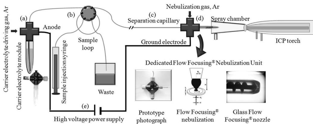
**Figure 1.** Scheme of the system prototype and photographs of some system components.
