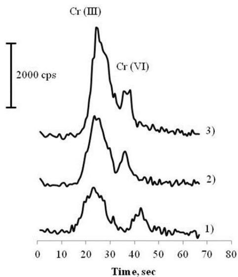
**Figure 4.** Influence of sample injection time on the Cr species separation. Sample Cr(III) and Cr(VI) 10 mg/L each; carrier electrolyte 15 mM HNO<sub>3</sub>; flow generating pressure: 1.5 bar; separation potential 14 kV; injection time: 1) 3 sec, 2) 4 sec, 3) 5 sec.
