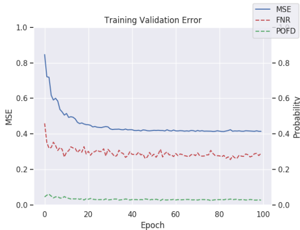
Figure 4: Evolution of the U-net MSE, FNR and POFD scores during training of the baseline model \lambda = 0, \mu = 0 using validation data.
