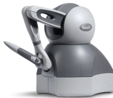
Figure 2.3: Geomagic Touch (formerly SensAble Phantom Omni), an affordable 3-DoF Haptic Device, used by the weDRAW Project.
