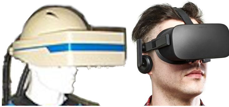
Figure 3.2: Left: First VR headset from VPL Research, which has been described as a “motorcycle helmet [with a] visor [that] is opaque and protrudes abruptly at eye level” (Wright, 1987) Right: modern VR headset (Oculus Rift).
