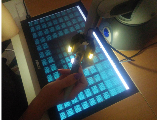
Figure 4.3: The Multisensory Addon: an addon for the Phantom Omni that produces sounds and emits light through two LEDs.
