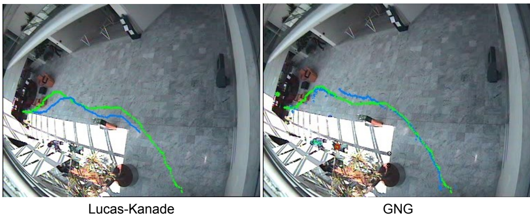
Figure 9: Estimated trajectory using GNG and Lucas-Kanade method in the WalkSplit video sequence. Left: Lucas-Kanade trajectory estimation. Right: GNG-based trajectory estimation. (Blue line: estimated trajectory. Green line: ground truth trajectory.)
