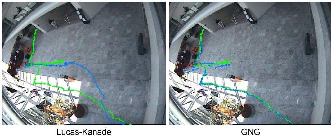
Figure 8: Estimated trajectory using GNG and Lucas-Kanade method in the MeetSplit3rdGuy video sequence. Left: Lucas-Kanade trajectory estimation fails due to pixel intensity similarities between different people moving around the scene. Right: GNG-based tracking method is able to correctly estimate the person trajectory. (Blue line: estimated trajectory. Green line: ground truth trajectory.)
