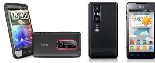
Fig. 2. Smartphones endowed with 3D camera. HTC EVO 3D (left) and LG Optimus 3D (right).
