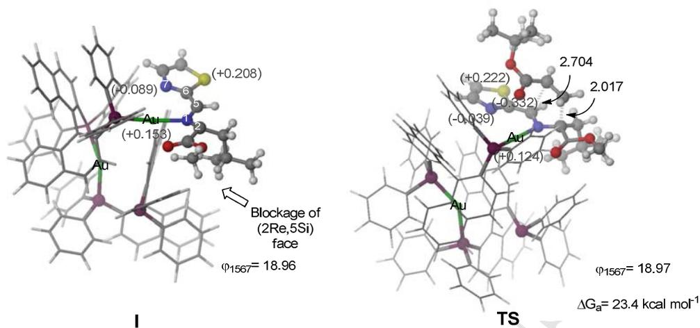
**Figure 7.** Gibbs activation energy and main geometrical features of the computed ylide and transition structures corresponding of the 1,3-DC of Au(I) ylide complex and *tert*-butyl acrylate computed at ONIOM(B3LYP/LanL2DZ:UFF) level of theory. High level and low-level layers were represented as ball & stick and wireframe models respectively. Grey numbers in parentheses represent Mulliken charges. Distances are in Å.
