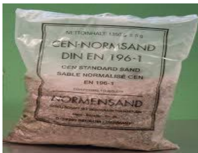
Figure 2 – Standard Sand EN 196-1
