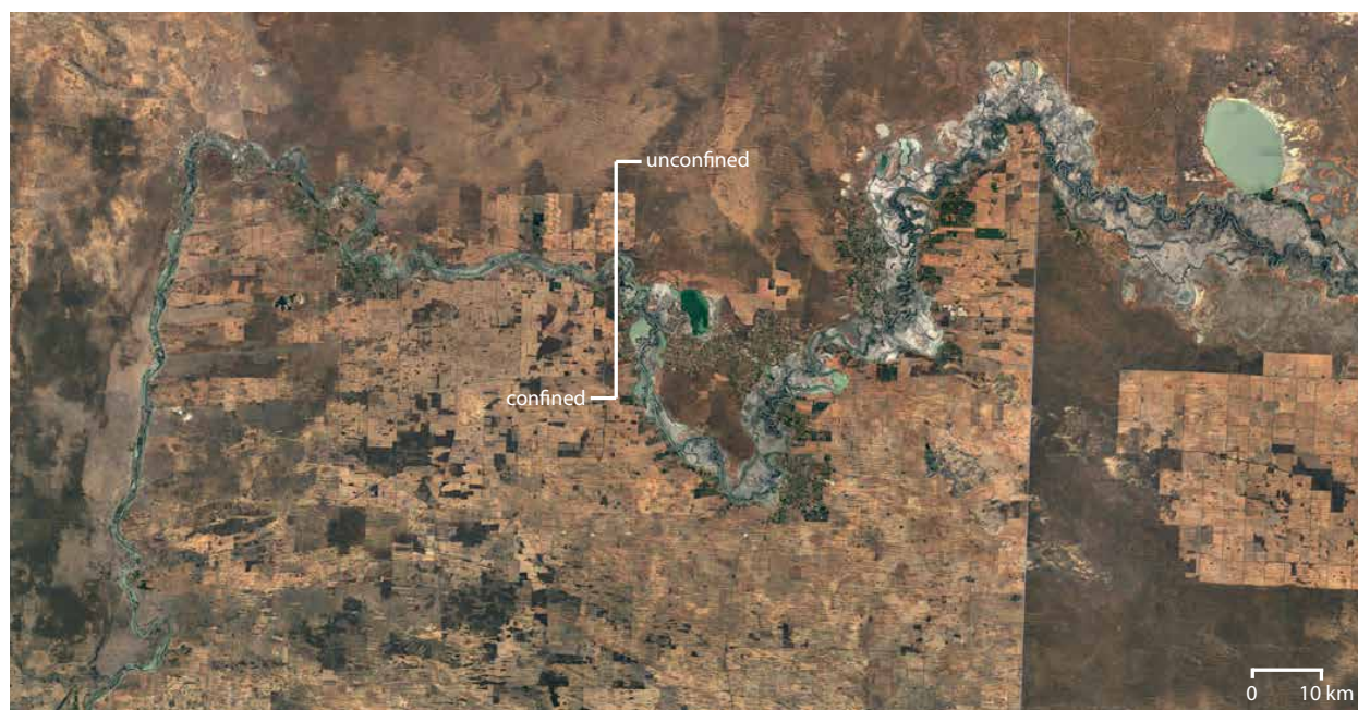
Figure 1.11: Satellite imagery showing the upstream extent of the Murray Gorge at Overland Corner. The lower Murray River enters the Murray Gorge at Overland Corner (rkm 439; white line). The dramatic transition in planform brought about by this confinement is strikingly apparent from satellite imagery. Satellite imagery source: Google Earth.
