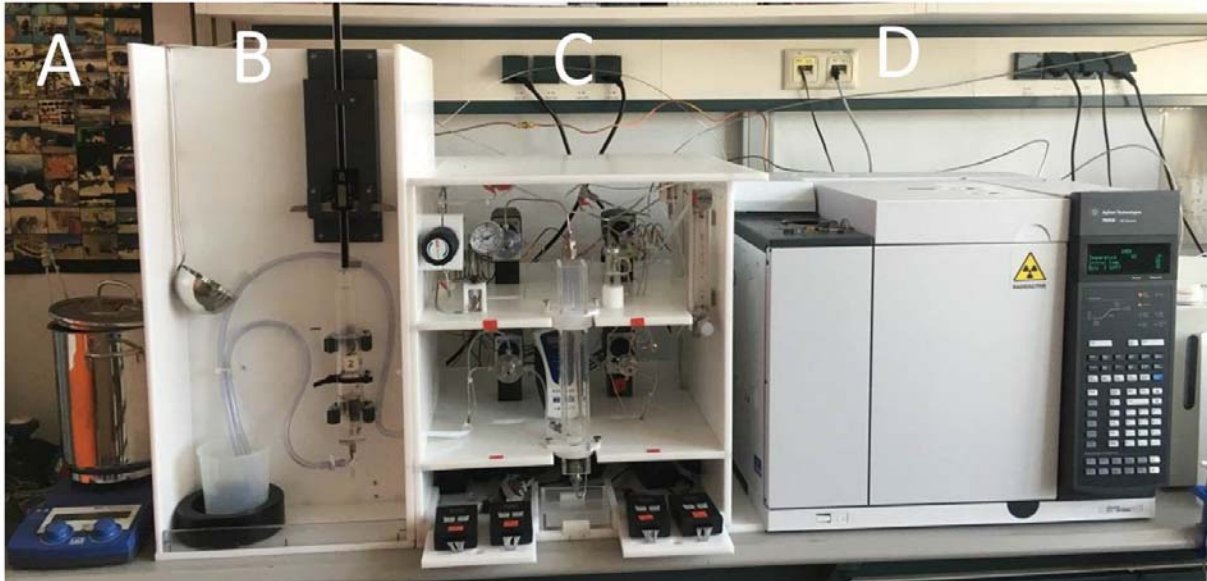
Fig. 5.3.4 The purge and trap system (IOW, Chemistry department). The system consists of four main components: A; the trap in the heating or cooling bath, B; Sample injection unit, C; Purge chamber with integrated frit and D; gas chromatograph.
