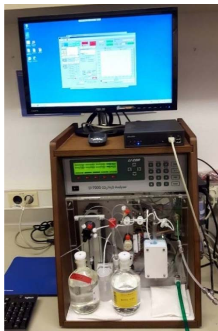
Fig. 5.3.6 Automated Infra-Red Inorganic Carbon Analyzer (AIRICA), IOW, Chemistry department.
