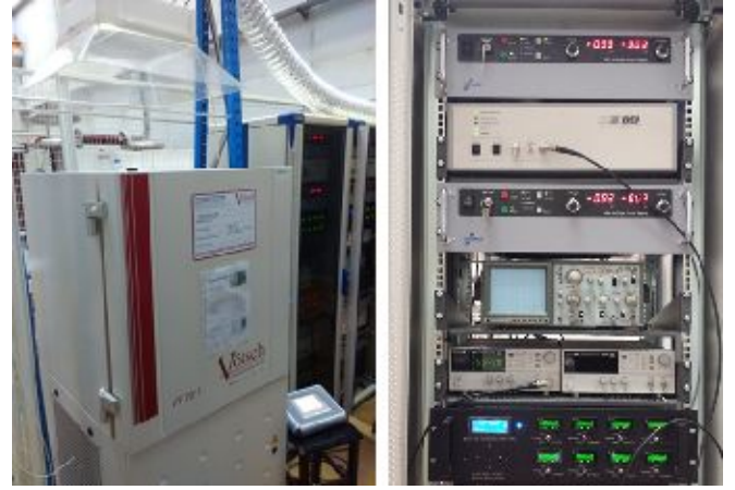
Fig. 5. The automatized test bench for the accelerated aging tests: climate chamber (left) and high voltage pulse generator with the lifespan counters (right)
