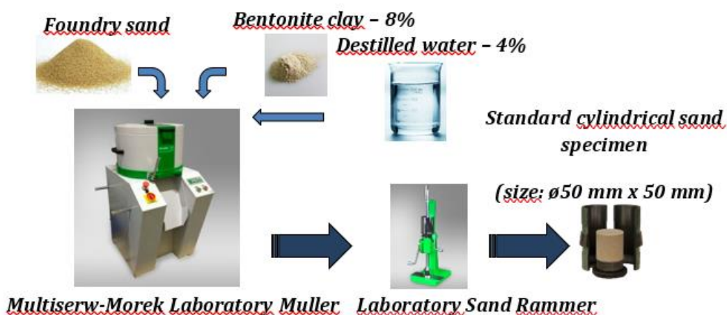
Figure 4. Process of making test specimens
