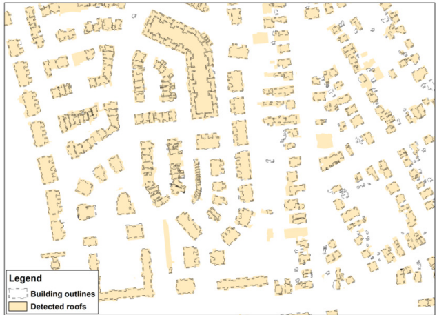
Figure 4: Comparison of roofs detected automatically and the official survey database.
