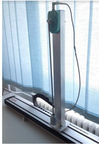
Figure 2. Inverted pendulum mounted on a Rexroth compact module
