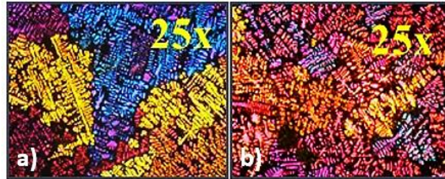
Figure 5. The Barker colour etched micrographs: (a) 3 rd alloy before grain refinement, (b) after the addition of AlTi5B1 grain refining master alloy
