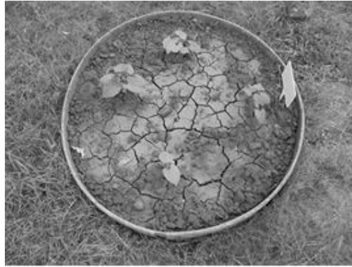
Figure 2. Arrangement of bean seedlings in a lysimeter
