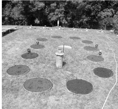
Figure 1. The simple drainage lysimeters involved in the experiment
