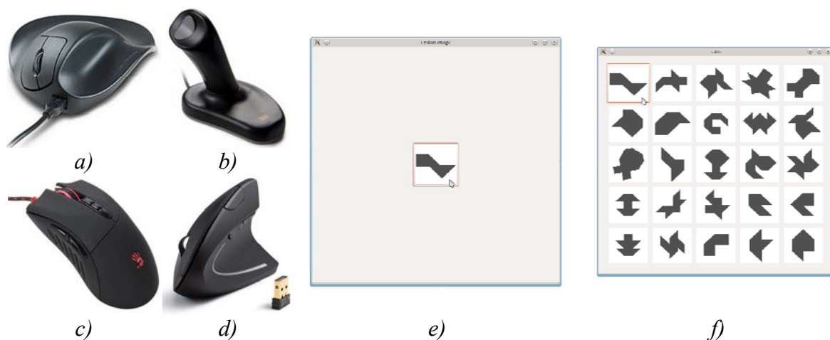
Figure 1 – Mice examined: A4Tech Bloody Ultra Gear mouse (a), Anker Vertical Ergonomic Mouse (b), Hippus Handshoe Mouse (c), Anir Vertical Mouse (d); The testing software (e, f)
