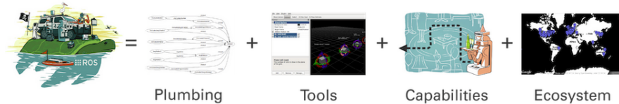
Figure 2.2: Plumbing: ROS provides publish-subscribe messaging infrastructure. Tools: ROS provides an extensive set of tools for configuring, debugging, visualizing, logging etc. Capabilities: ROS provides a broad collection of libraries. Ecosystem: ROS is supported and improved by a large community, thousands of ROS packages [1]
