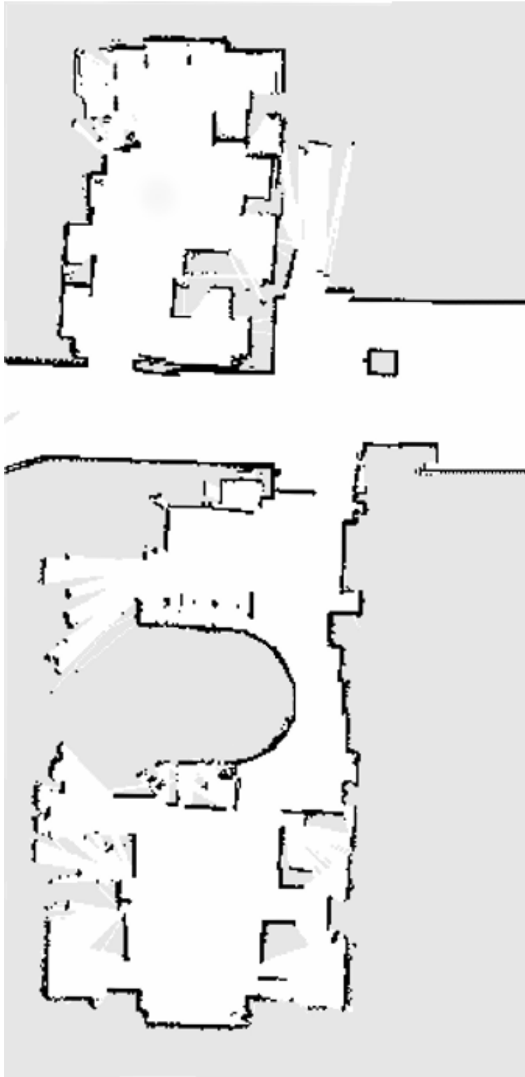
FIGURE 2.9: Map of the robot's workspace used during the experiments, obtained using SLAM.
