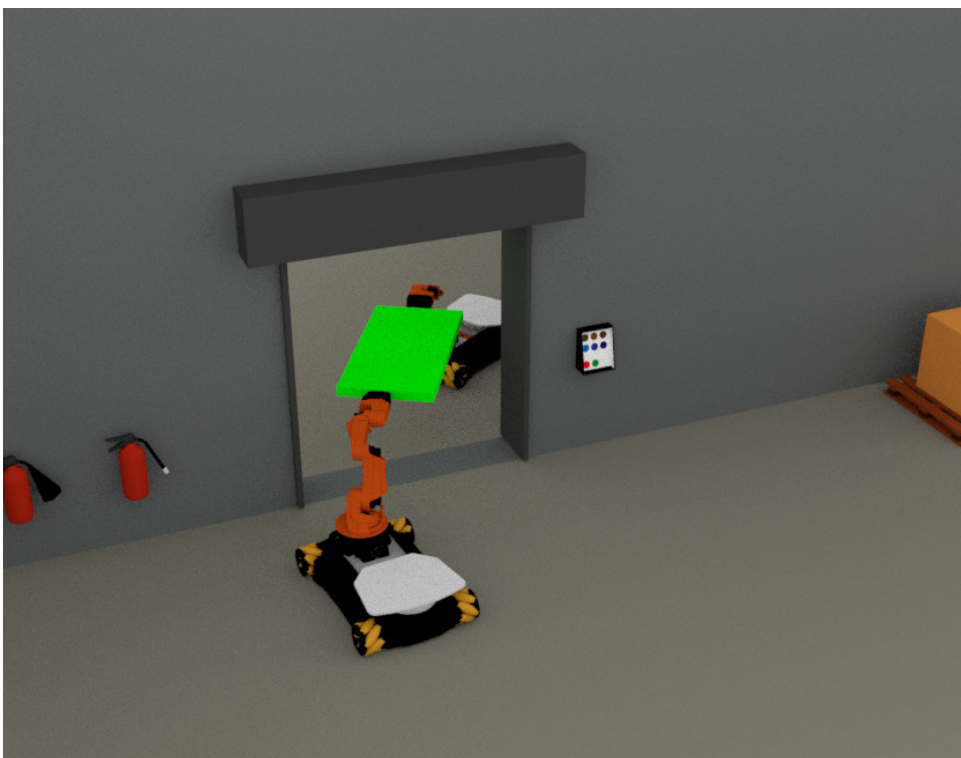
FIGURE 5.1: Cooperative object transportation by two robots.
