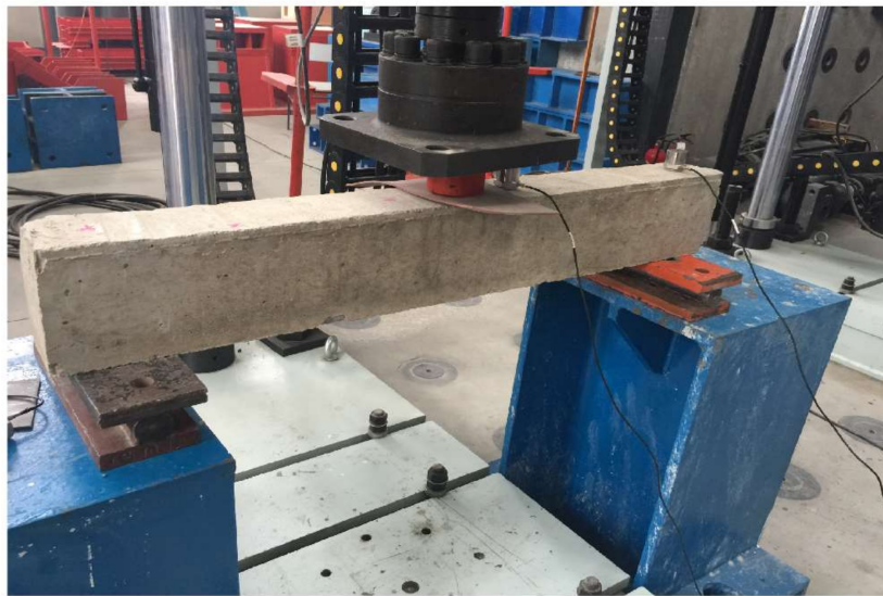
Figure 7. (a) Illustration of test setup with reinforced concrete beam and (b) photograph showing experimental setup. Dimensions in (mm).
