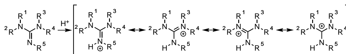
Scheme 1.9: Protonation of an arbitrary guanidine and the delocalization of the positive charge on the guanidinium cation.
