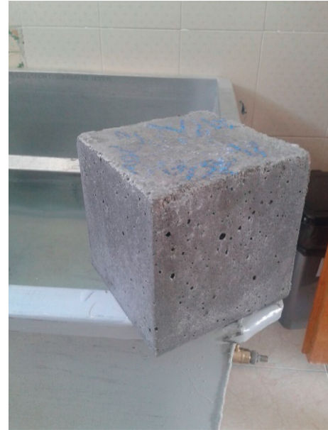
FIGURE 6: One of the normal concrete samples (without granite aggregates) after 24 hours of curing in water.
