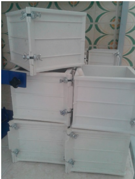
FIGURE 5: The used plastic. The plastic was chosen for better quality of samples and to avoid sticking.
