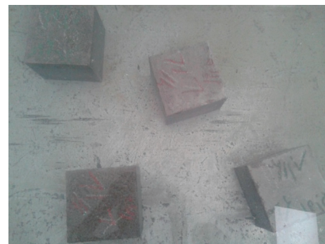
FIGURE 7: The soaked samples which are controlled by the digital temperature controller at 30°C for the first 24 hours.
