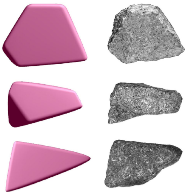
Fig. 11 Real ballast and corresponding polyhedron simulated ballast [164]
