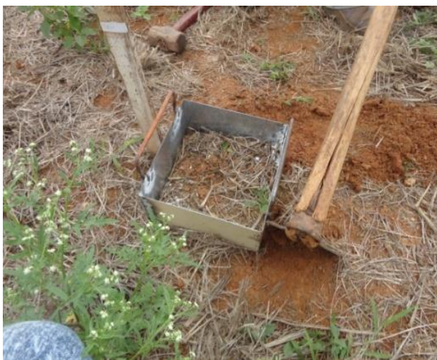
Figure 3. Representation of the template on the ground (A) at the desired depth and template removal with a trench shovel (B). This process was carried out in the maize crop, with conventional treatment and organic treatment, in the area belonging to Embrapa Maize & Sorghum, in the municipality of Sete Lagoas, MG.
