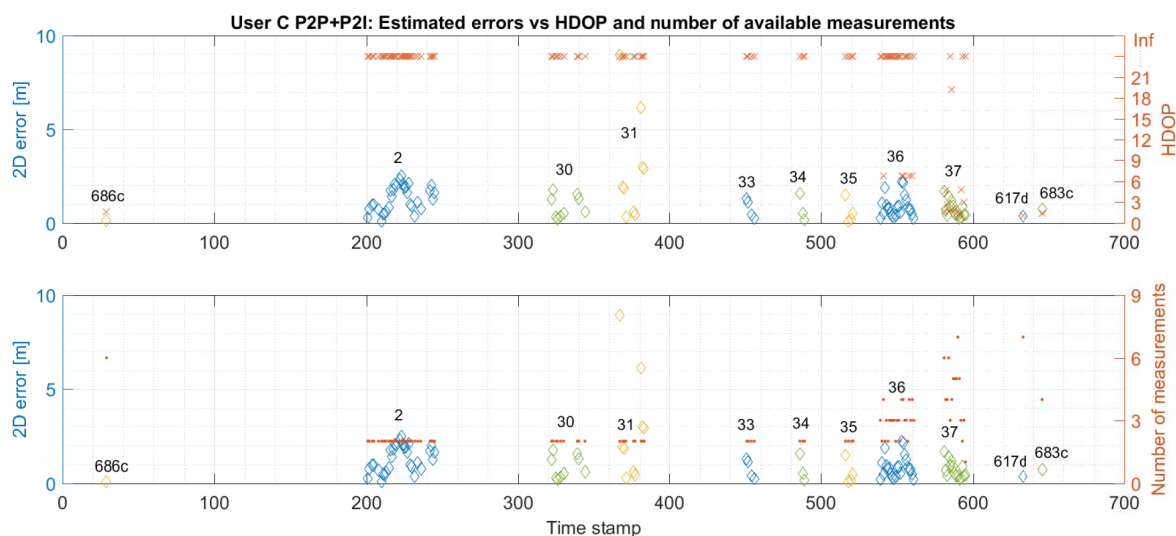
Figure 17. Comparison of estimated errors at each checkpoint with respective values of HDOP (upper graph) and the number of available measurements (bottom graph) for trajectory S1–I1–S2 for User C. Positions are estimated using Pozyx UWB and User Z's data (P2P+P2I EKF).
