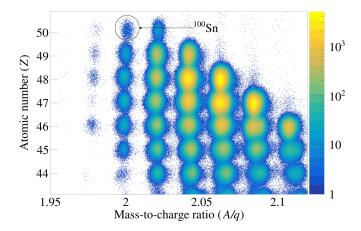
FIG. 1. Particle identification plot of proton-rich radioactive nuclei produced in this experiment. <sup>100</sup>Sn is marked as a reference.
