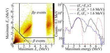
FIG. 2. Left: maximum energies deposited in x- and y-side DSSSD strips for decays correlated to  ${}^{97}$ Cd implantation events. The void where 3.5 < E (MeV) < 6.0 on the x-side strips is due to an ADC saturation of the x-side strip channels, resulting in overflow events appearing at E > 6 MeV. Right: energy projections of the 2D matrix on the left. See Sec. II E for details.
