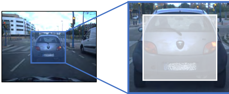
Figure 6.5: Area considered by the proposed object localization approach within an object's bounding box
