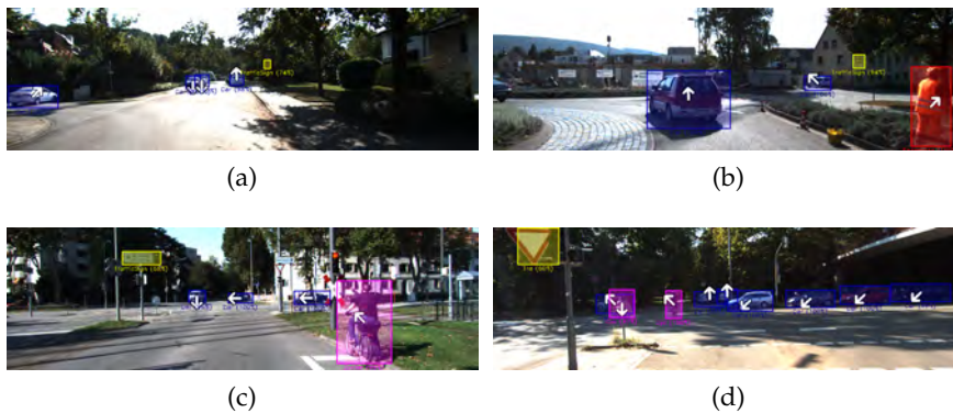
Figure 5.18: Selected examples of object detection and viewpoint estimation results on the KITTI test dataset with additional categories [115] © 2018 IEEE
