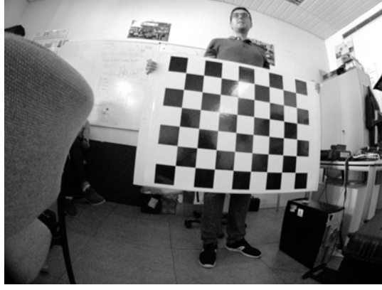
Figure 3.5: Checkerboard pattern used for intrinsic calibration as seen from a camera with a high positive radial distortion (barrel distortion)
