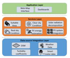
(a) Scheme of the software architecture for PV systems integration into Smart Grids
