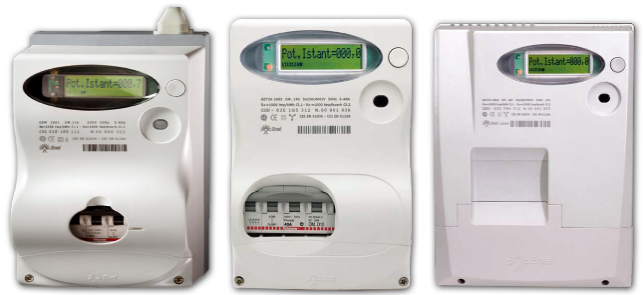
Figure 4. Smart meters used for Telegestore – from left to right: single phase (GISM), poly phase meter for demand up to 30 kW (GIST), poly phase meter with current transformer (CT) for demand up to 200 kW (GISS).
