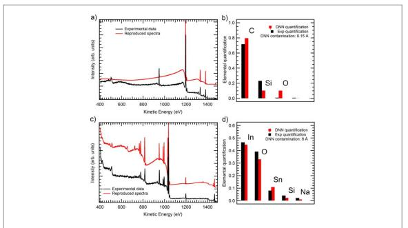
**Figure 6.** Application examples on two experimental sets; spectra (a) and quantification  $q_i$  (b) for carbon nanotubes on Si; spectra (c) and quantification  $q_i$  (d) for indium-tin oxide (ITO) deposited on Si. For the ITO case, the adventitious carbon contamination was factored out from the experimental quantification.
