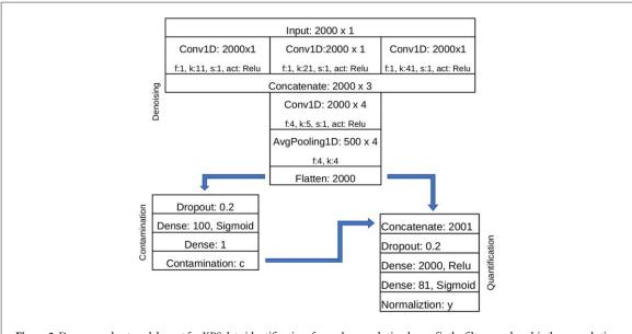
**Figure 3.** Deep neural network layout for XPS data identification; for each convolution layer, f is the filter number, k is the convolution kernel size, k is the stride length. Total number of trainable parameters is 4366 410.
