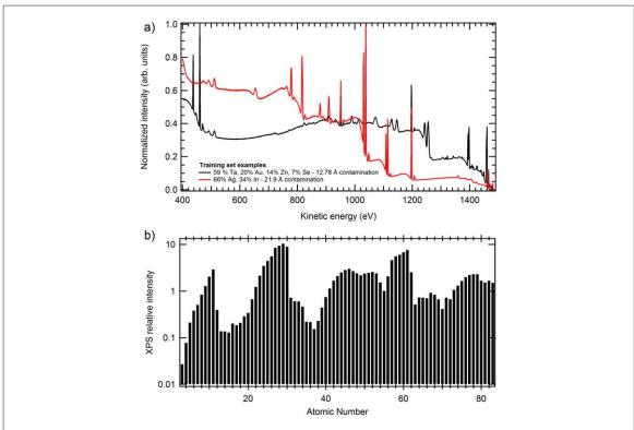
Figure 2. (a) An excerpt of two simulated survey training spectra, (b) maximum XPS intensity  $(T_i)$  of simulated spectra for each pure element, calculated for a fixed photon flux. Photon energy is 1486.6 eV, and KE spectra range is 400–1486 eV.
