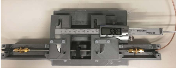
Figure 5: Experimental setup employed for transmission-based dielectric measurements. The two open-ended coaxial-cables are embedded in a plastic support and connected to a 2-port VNA (not shown in the figure). A caliper serves to measure the separation distance between the probes. Between the probes, a phantom is measured.
