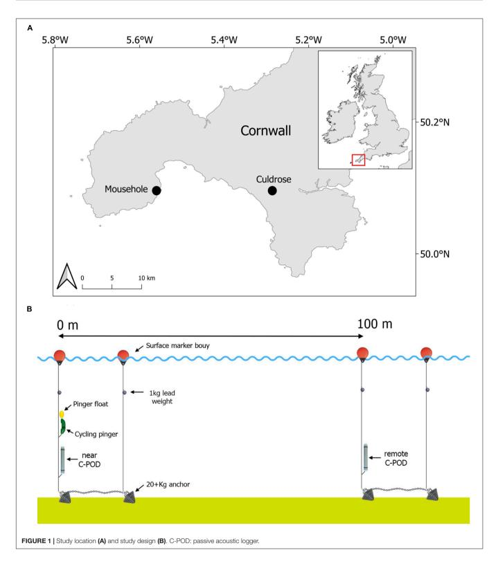
throughout the study to measure the effects of the pinger (Tregenza et al., 2016). The near C-POD ceased recording on March 17th 2013 at 02:00 (229 days of records) and was subsequently retrieved. A second C-POD was deployed on November 8th 2012 at 17:00, 100 m away from the pinger,
