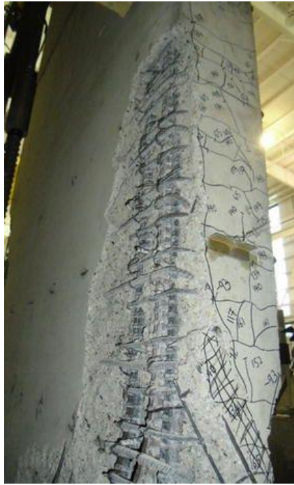
Figure 13 – Splitting in specimen by Villalobos (2014, 2017).
