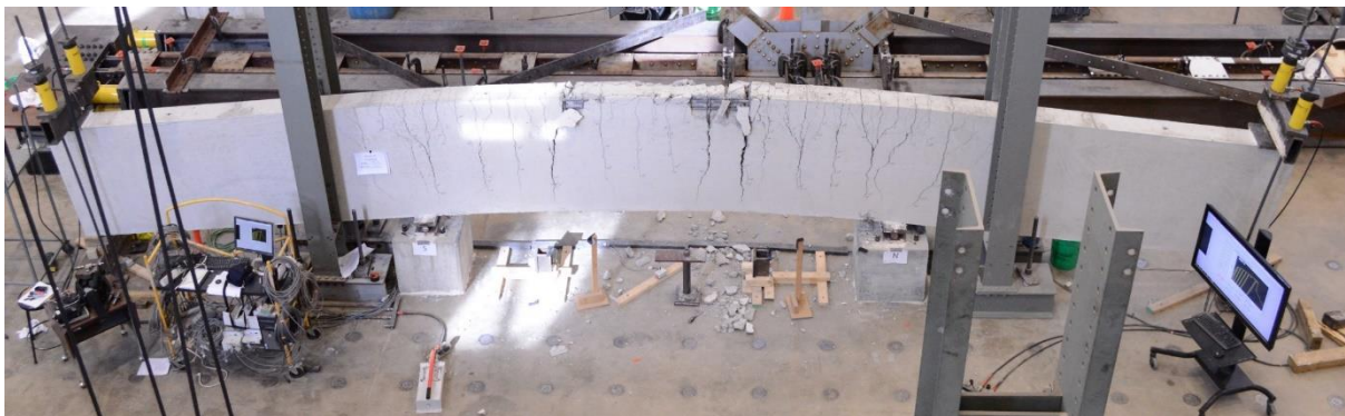
Figure 19 – Four-Point Bending Test Setup – Lap Splice Visible at the Top of the Beam at Midspan.
