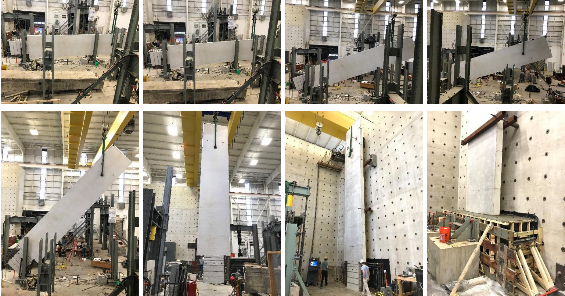
Figure 47 – Wall tilting process and foundation fabrication.
