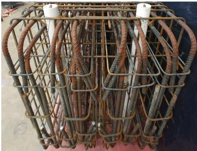
Figure 27 – Reinforcement in Wall Foundation – Confinement of End Hooks.
