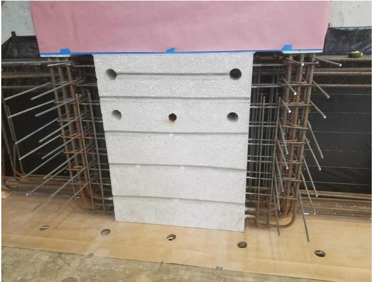
Figure 44 – Shear keys, steel bushing, and openings in supporting stub of test walls.
