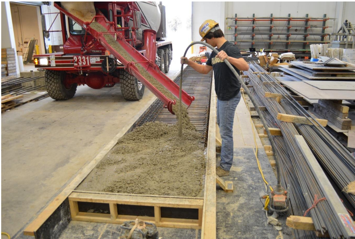
Figure 38 – Casting of Test Beam.
