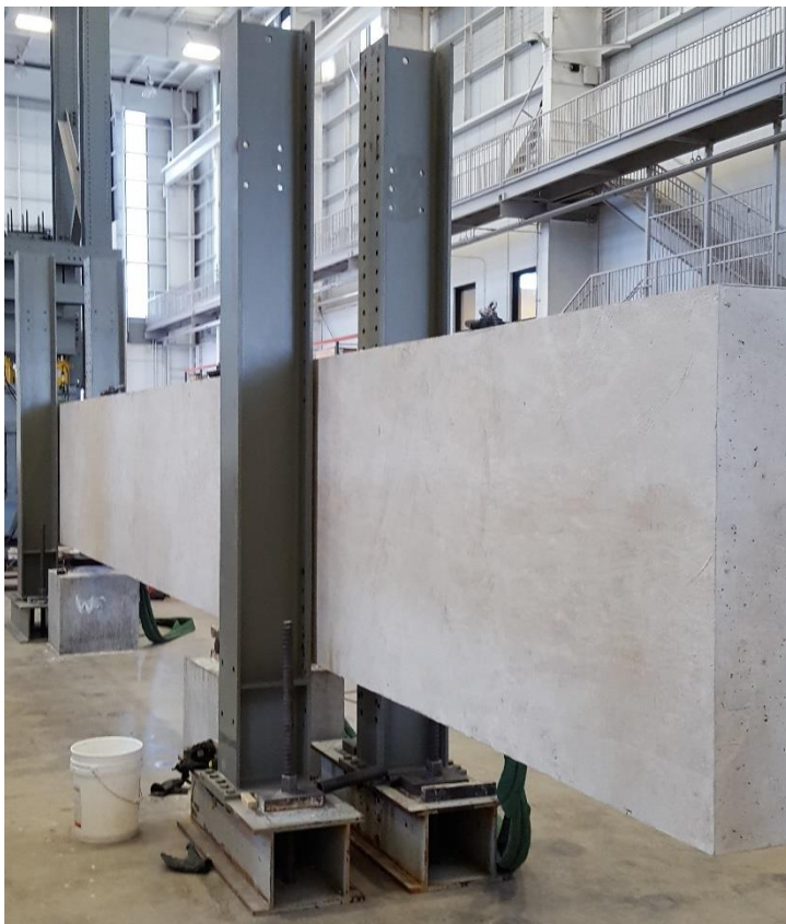
Figure 41 – Bracing used in Four-Point Bending Tests of Beams.
