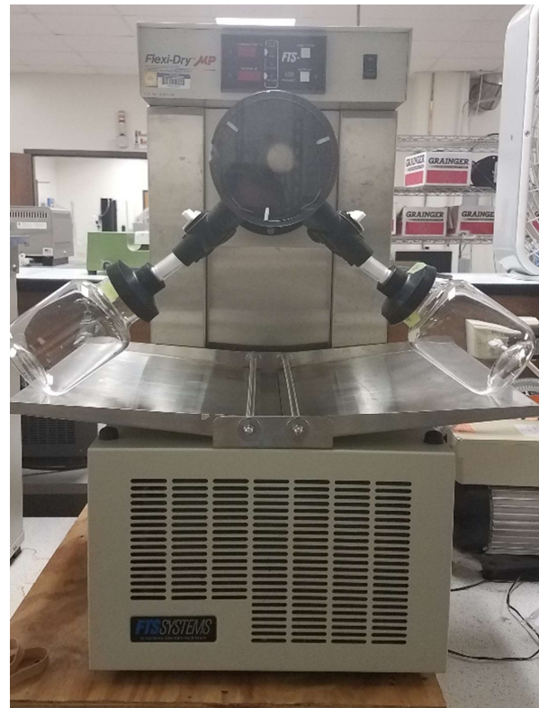
Figure 3: Freeze-drying apparatus used to lyophilize CFPS systems.
