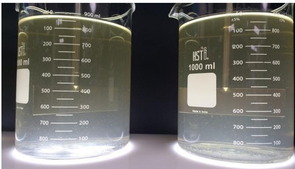
Figure 14. White precipitates visible in jars after completion of the precipitation test
