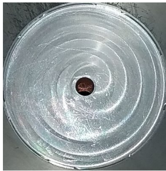
Fig. 8 Misalignment of cryogenic shroud initially eclipsed apertures
